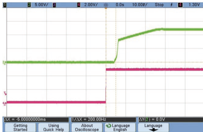
Fig. 12-3: On/Off Enable Delay (CH2: Vout; CH4: Enable) Ta=+25°C, Vin = 12V, Iout = 0A, Load = 200μF
