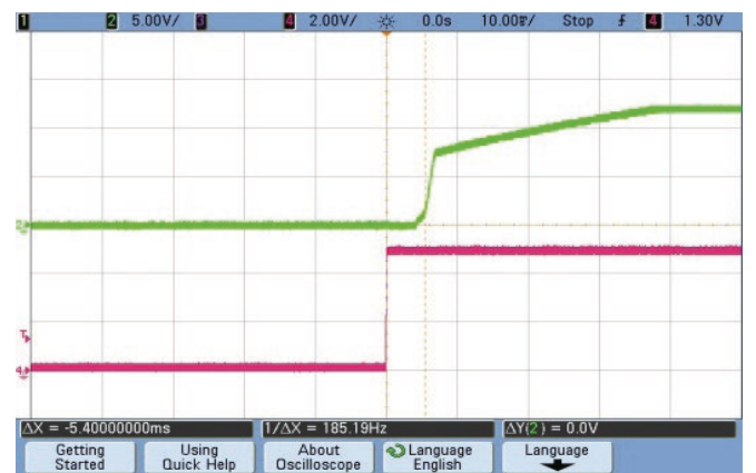
Fig. 12-4: On/Off Enable Delay (CH2: Vout; CH4: Enable) Ta=+25°C, Vin = 12V, load = 10A, Load = 4700μF
