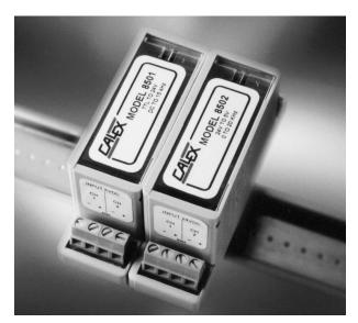
**Model 8501** is a two channel converter, 5V to 24V. The two independent channels require 7mA into 382 ohms to provide a 7mA output into the 3K, 24 volt typical PLC logic inputs. They may be driven by standard or H series TTL logic, or with an open collector NPN transistor. Note that low power TTL logic will not drive this unit. The output is a floating optocoupler NPN transistor which may be connected in either a source or sink configuration. The input frequency range is DC to 15KHz.
