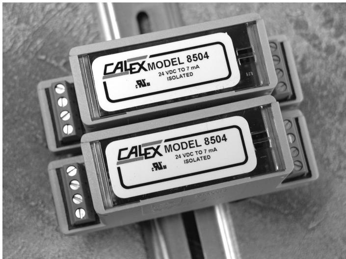
**Model 8503 and 8504** Dual Channel PLC Interface modules are designed to interface 120 Volt AC line or 24VDC signals to the PLC 24 Volt, 7mA discrete inputs. The inputs are isolated from the outputs by an optocoupler and the two channels are independent. Power is supplied by the input signal and is a nominal 10mA per channel. The output transistor is fully floating allowing either source or sink connection to the PLC.
