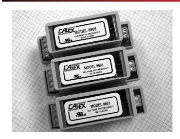
**Model 8605, 8606, 8607** analog input modules are designed to interface with the 24 VDC logic inputs for applications requiring additional analog inputs. The 8600 modules output a square wave up to 500 Hz allowing the PLC to count the frequency producing about 8 bit resolution, 1 part in 500.
