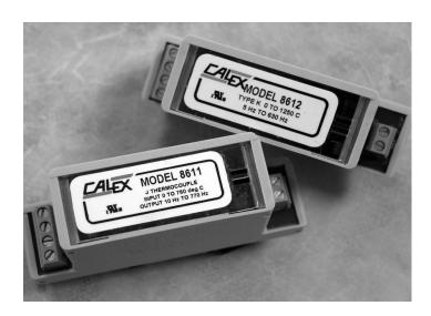
**Model 8611** Type J thermocouple to frequency converter is designed to operate into the common 24 Volt, 7 mA PLC inputs. It's output is an isolated optocoupler transistor and provides DC isolation from the input and DC power. The 8611 will operate with a DC supply of 15 volts to 26Volts at 17 mA
