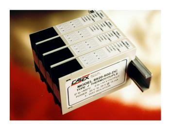
The 8900 Series offers a low cost TC (thermocouple) and RTD signal conditioning solution for applications that require a 0-10V output signal. All models isolate and linearize. The thermocouple conditioners also have cold junction compensation. The 8900 Series also offers a variety of analog to analog isolators, i.e. 0 - 50 mV to 0 - 10 V or 4 - 20 mA to 0 - 10 V etc. The isolation is three way, input to output, input to power and output to power. All models are powered by 24 VDC.
