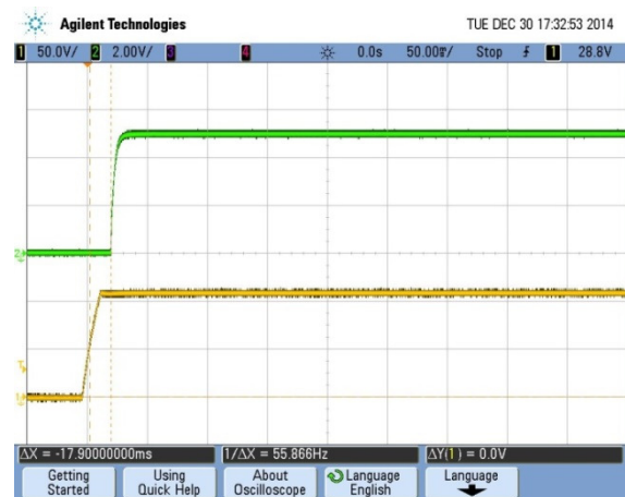
Turn-on transient at full load current (50 mS/div, Top Trace: Vout, 2V/div; Bottom Trace: Vin, 50V/div)
