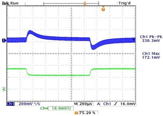
Step Load Transient Response ( $V_{in}=24V$ ,  $V_{out}=\text{nom.}$ ,  $I_{out}=50-75-50\%$  of full load,  $C_{load}=2000\mu F$ ,  $T_a=+25^\circ C$ ., ScopeBW=20MHz)
