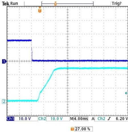
On/Off Enable Delay (Negative logic,  $V_{in}=24V$ ,  $V_{out}=nom.$ ,  $I_{out}=2A$ ,  $C_{load}=0\mu F$ ,  $T_a=+25^{\circ}C.$ , ScopeBW=20MHz) Trace 1=Enable, Trace 2=Vout
