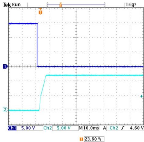
On/Off Enable Delay (Negative logic, Vin=24V, Vout=nom., Iout=4.5A, Cload=0 μF, Ta=+25°C., ScopeBW=20MHz) Trace 1=Enable, Trace 2=Vout
