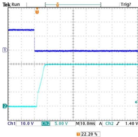
On/Off Enable Delay (Negative logic,  $V_{in}=24V$ ,  $V_{out}=nom.$ ,  $I_{out}=3.3A$ ,  $C_{load}=0\ \mu F$ ,  $T_a=+25^{\circ}C.$ ,  $ScopeBW=20MHz$ ) Trace 1=Enable, Trace 2=Vout
