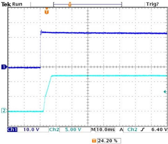
Power On Startup Delay ( $V_{in}=0$  to  $24V$ ,  $V_{out}=\text{nom.}$ ,  $I_{out}=4.5A$ ,  $C_{load}=0\mu F$ ,  $T_a=+25^\circ C$ ., ScopeBW=20MHz) Trace 1= $V_{in}$ , Trace 2= $V_{out}$
