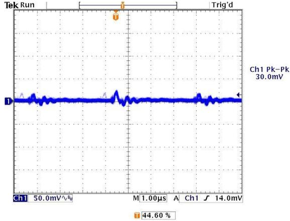
Output Ripple and Noise ( $V_{in}=24V$ ,  $V_{out}=nom.$ ,  $I_{out}=3.3A$ ,  $C_{load}=1\mu F\ ceramic\ II\ 10\mu F\ tantalum$ ,  $T_a=+25^{\circ}C.$ ,  $ScopeBW=20MHz$ )
