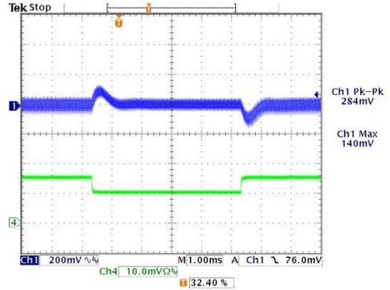
Power On Startup Delay ( $V_{in}=0$  to  $24V$ ,  $V_{out}=nom.$ ,  $I_{out}=no$  load,  $C_{load}=0\mu F$ ,  $T_a=+25^\circ C.$ , ScopeBW=20MHz) Trace 1= $V_{in}$ , Trace 2= $V_{out}$
