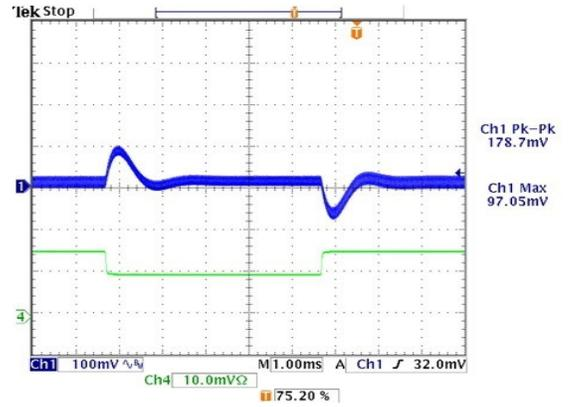
Power On Startup Delay ( $V_{in}=0$  to  $24V$ ,  $V_{out}=\text{nom.}$ ,  $I_{out}=\text{no load}$ ,  $C_{load}=0\mu F$ ,  $T_a=+25^\circ C$ ., ScopeBW=20MHz) Trace 1= $V_{in}$ , Trace 2= $V_{out}$
